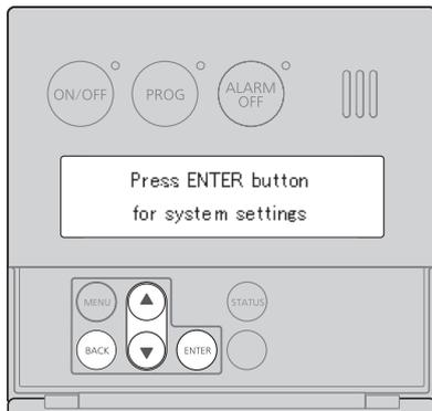
Note: When power is first connected to the multi-unit system (system controller and units), the remote enters an initial setting mode. The following instructions explain how to perform an initial setting. If you need to change these settings at a future date, follow the instructions titled System Selection and Settings in the “Initial Settings” Screen (page 10 - 12).
