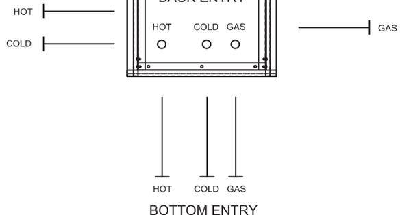
Note: Allow for drainage from the pressure relief valve.
